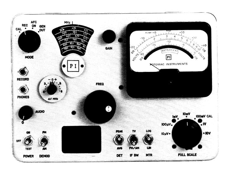
Figure 2-1. Operating Controls and Indicators
